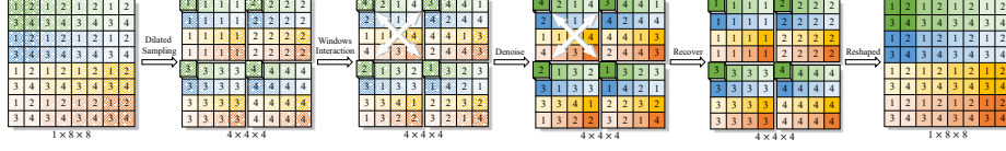
Fig. 5: Illustration of dilated sampling with window interaction: 8 \times 8 higher-resolution and 4 \times 4 low-resolution. The number \{1, 2, 3, 4\} represent the different positions within the same window (same color). The interaction operation is conducted in the window.
