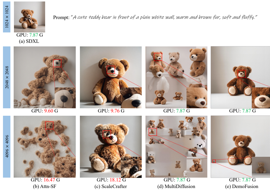
Fig. 1: Comparison of image quality and GPU overhead for existing higher-resolution generation methods. The GPU memory of Attn-SF [12] and ScaleCrafter [6] significantly increases with resolution, while patch-wise denoising methods, e.g. , MultiDiffusion [1] and DemoFusion [4] suffer object repetition issue. Best viewed zoomed in.
